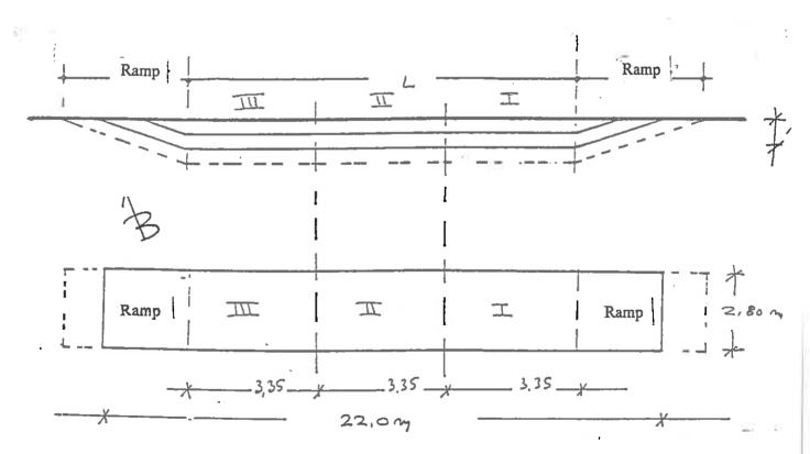
The test embankment was layed inside a pit with dimensions 22.0 m X 2.80 m. The embankment was divided into three parts with three different material classifications in order to inspect the suitability of the different classifications.
